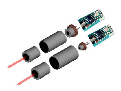
To get the LD mounted, you need to glue it into the holding fixture.
