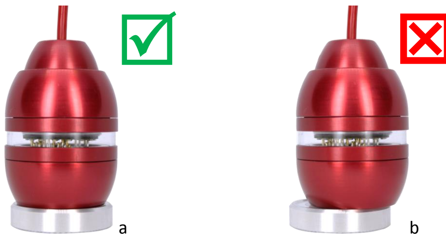
Fig. 5. Minispectrometer orientation relative to the etalon at calibration measurement: a – correct, b - incorrect.
